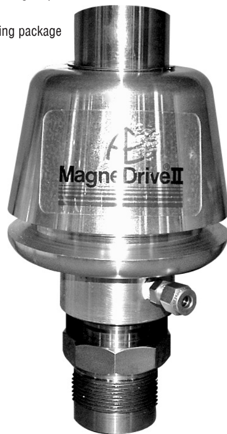
Outer magnets are rotated by a direct coupled motor, thus rotating inner magnets and rotor shaft.
