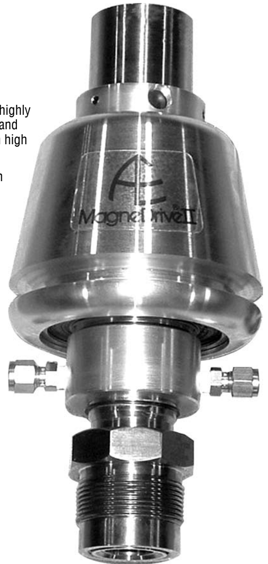
Outer magnets are rotated by a motor driven belt thus rotating inner magnets and rotor shaft.
