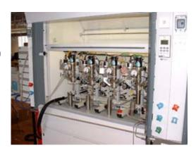
Multi-Reactor Systems: ▶Laboratory Reaction Systems Laboratory reactor system simulates production chemical processes
